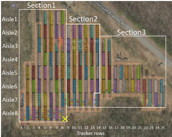
Fig. 4. Sketch of layout sections. The 1-layout model combines Sections 1, 2, and 3; the 2-layout model uses Section 1 as-is and combines Section 2 and 3; the 3-layout model uses each section as-is. Section 1 (54 strings), Section 2 (30 strings), Section 3 (27 strings).
